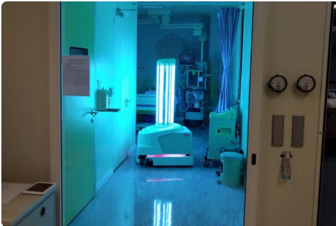
UVD disinfectant robot spreads ultraviolet rays in hospitals to kill bacteria and viruses
